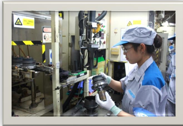
Searcher Jig Setting Pipe Fitting
